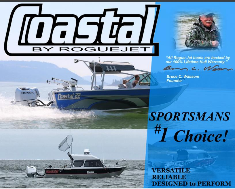
Decades of engineering, field testing and customer feedback has produced the Rogue Jet Boatworks "Coastal Series", designed for the sporting enthusiast. The progressive dead rise of the boats bottom from 18 degrees at the transom to 50 degrees at the bow, in combination with our signature full width outboard bracket and high sides for safety, has turned the Coastal into the Elite Sportsman's Choice.
